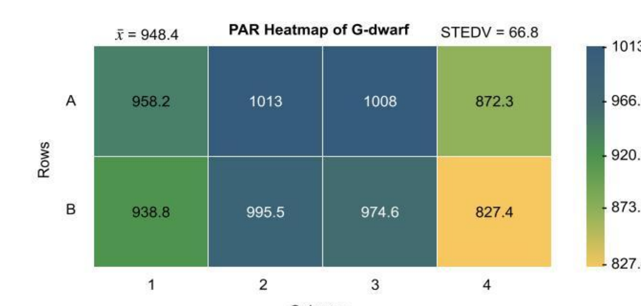
Figure 6: Heatmap of Photosynthetically Active Radiation (PAR) intensity across plastic table surface of the vivosun at 100%.
